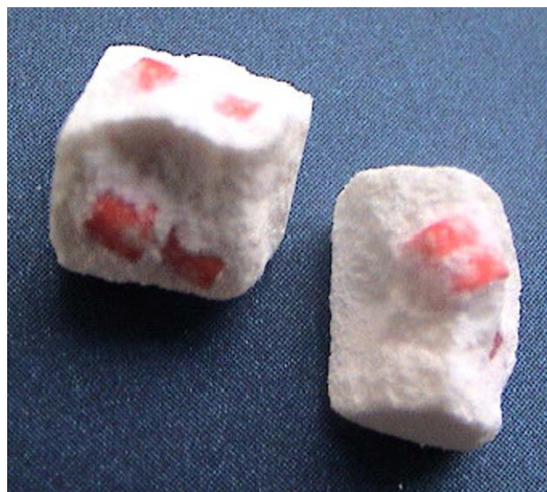
Fig. 2. Fracture equatorial showing surfaces of the compressed EC mini-tablets system.
